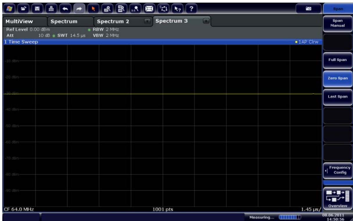
Fig. 4-7: Time domain display of the calibration signal
